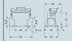
**N.B.:** the enclosures ensure IP66 protection rating when mated and locked with the closing levers.
